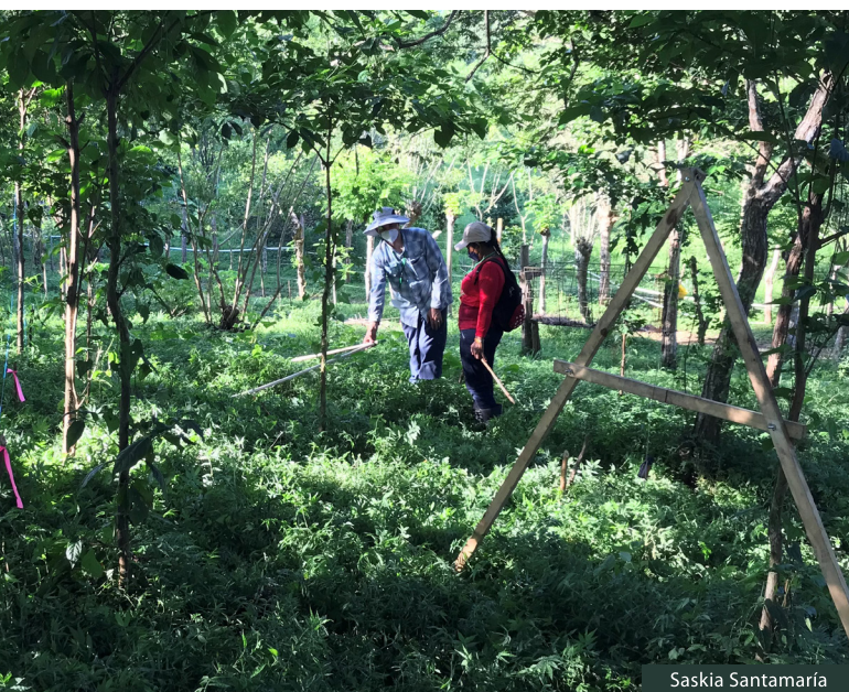
Participants practice measuring contour lines with an A-level.
